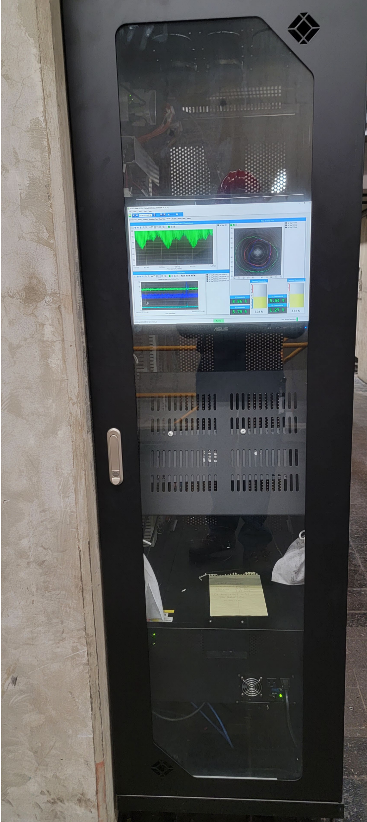
Figure A 4 MCM2 System with the Viewer application displaying rotor eccentricity information during operation.
