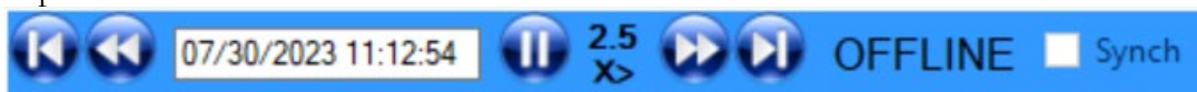
Figure 5 MCM2 Viewer Timebase in historic or offline playback mode - playing forward in time at 2.5x the original recorded speed.
